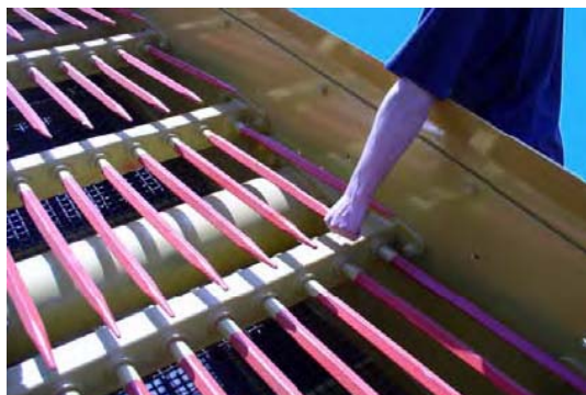
1: Check tine by shaking it as shown.
