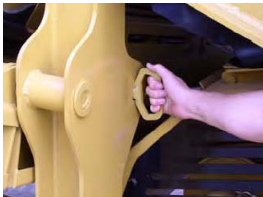
13: Remove mid grade side conveyor bottom section locking pins.
