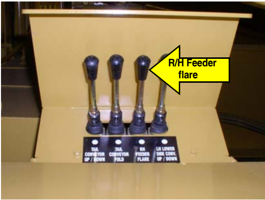
1: Activate 'R/H Feeder Flare' lever.
