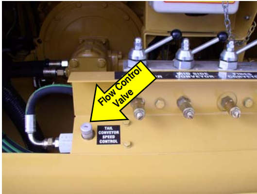
3: Adjusting Tail Conveyor
