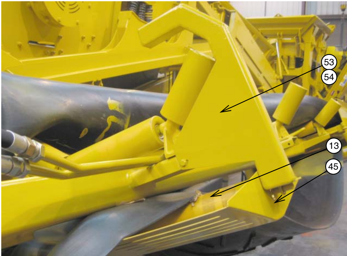
7: MID GRADE SIDE CONVEYOR RETURN ROLLERS
