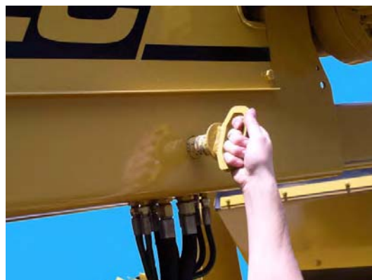
11: Replace locking pins.
