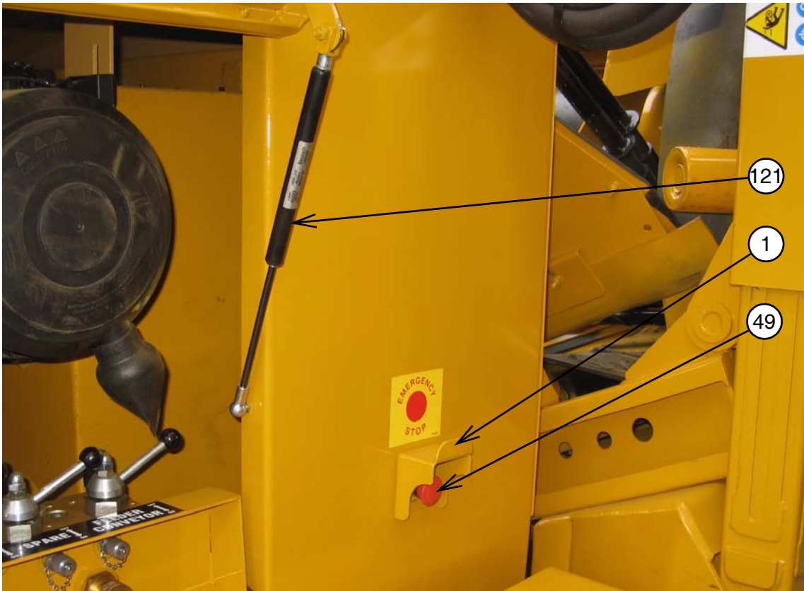
3: VIEW ON EMERGENCY STOP AND FLOW CONTROL
