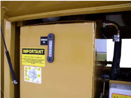
9: Check hydraulic oil level.
