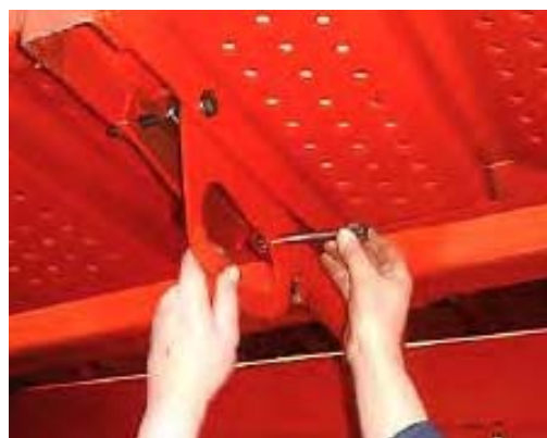
6: Insert pins & retain with R-clips to lock the walkway.
