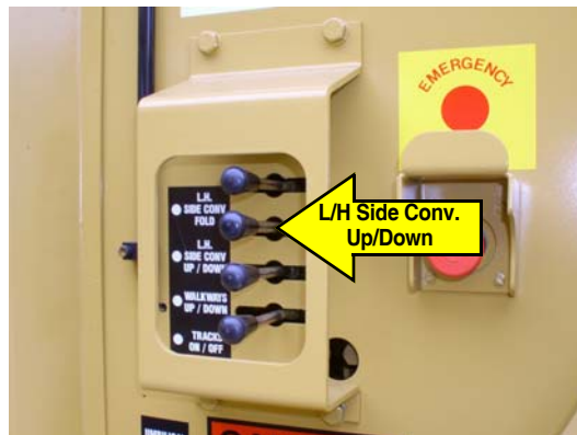
8: Activate 'L/H Side Conveyor Up/Down' lever to lower conveyor away from side of machine.
