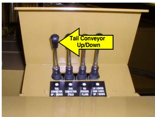
6: Activate 'Tail Conveyor Up/Down' lever to lower tail conveyor onto chassis.
