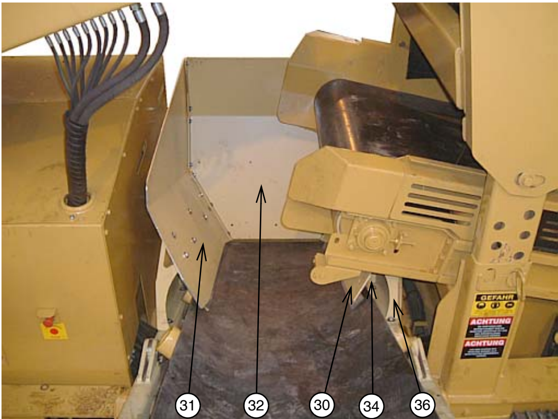
6: FINES SIDE CONVEYOR FEED BOOT
