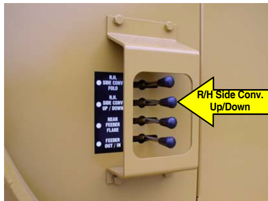
2: Activate 'R/H Side Conveyor Up/Down' lever to lower conveyor away from side of machine.
