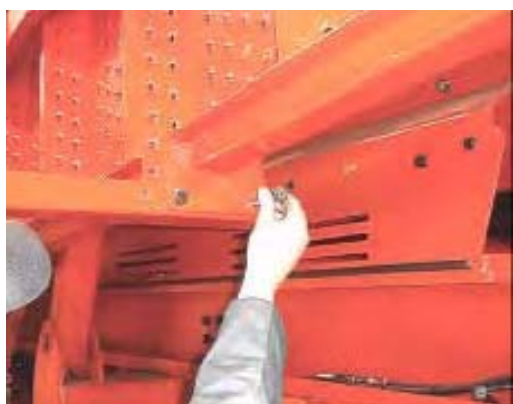
3: Re-insert pin & R-clips to lock out handrail.
