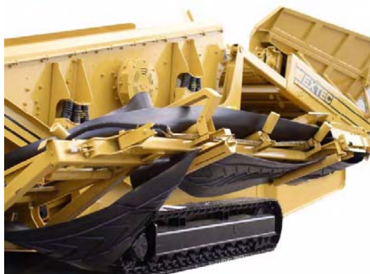
9: L/H Side Conveyor folded down
