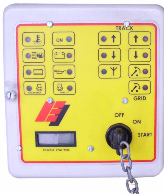
Figure 4-3: Electrical Control Box with Key
