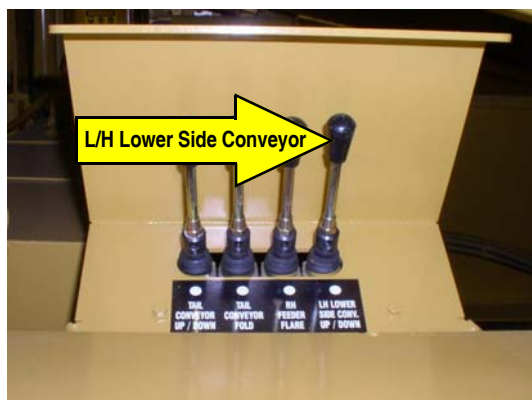
14: Activate 'L/H Lower Side Conv' lever to lower the mid grade side conveyor bottom section.
