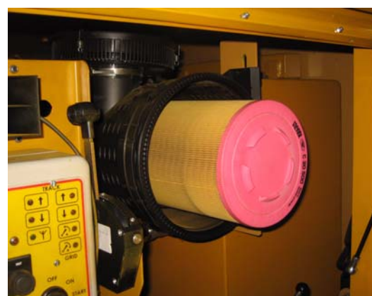
8: Loosen clips & remove outer element. EN9320
