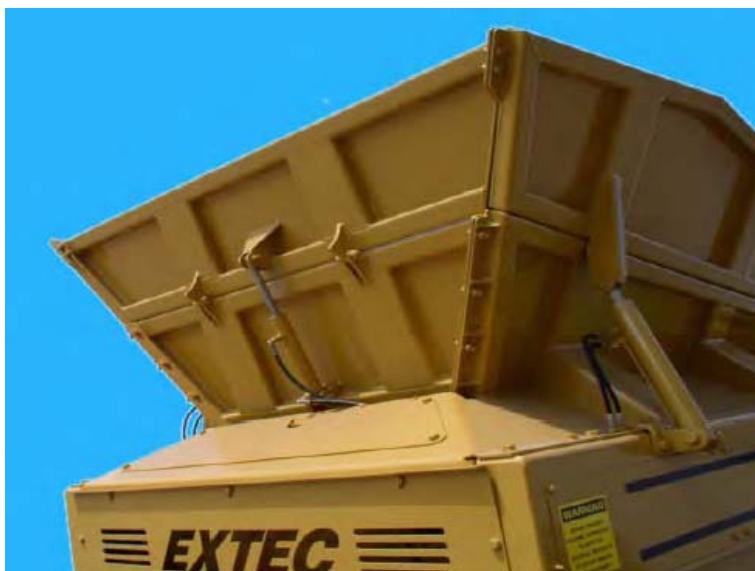
7: Bolt rear flare to both side flares and tighten.
