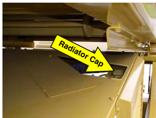
6: Check coolant level and refill if necessary. Use a 50/50 mixture of anti freeze and water.
