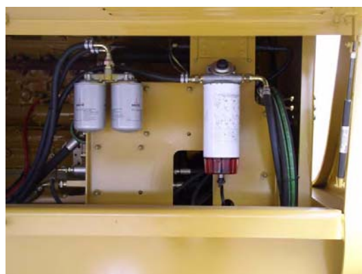
4: Bleed diesel water trap. EN7896
