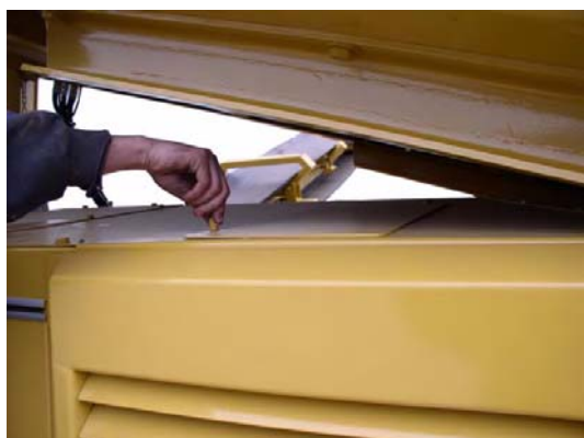
5: Remove radiator service guard.
