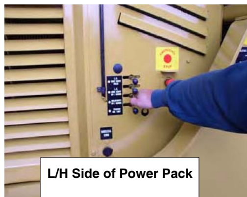
4: Activate 'Walkways Up/Down' lever to erect the walkways.
