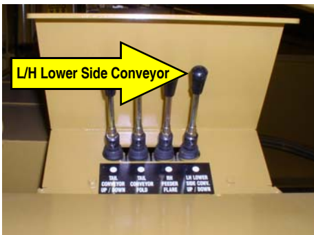
2: Activate 'L/H Lower Side Conveyor Up/Down' lever to raise the conveyor bottom section.
