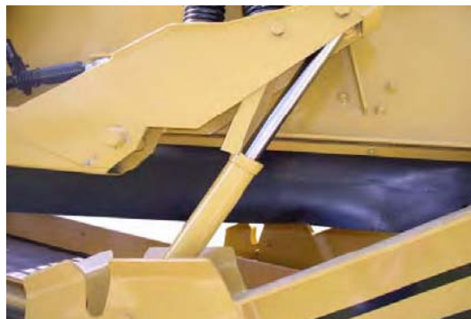
5: When finished, remember to release both lock-out legs before lowering screen box.
