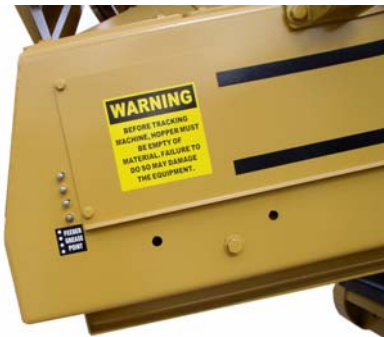
1: Feeder bulkhead grease point
