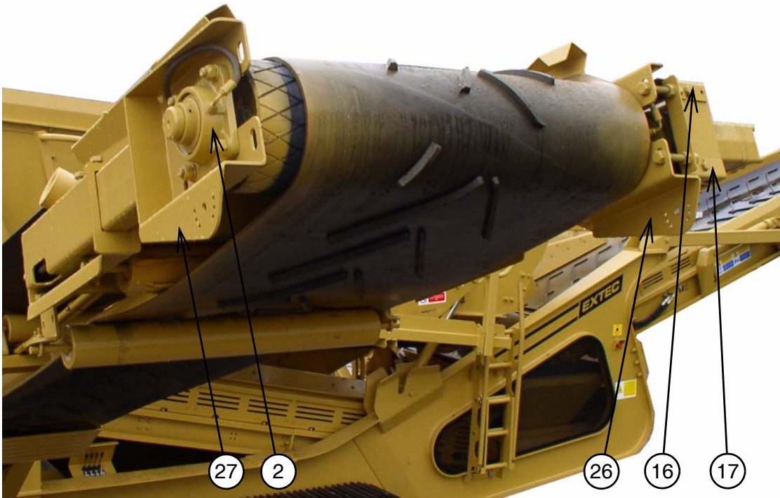
2: FINES SIDE CONVEYOR DRIVE END
