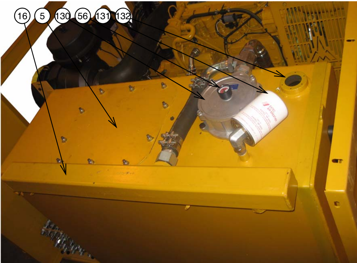
15: DETAILED VIEW ON HYDRAULIC TANK
