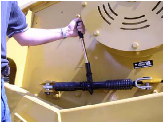
11: Check condition of screen mesh and tension.
