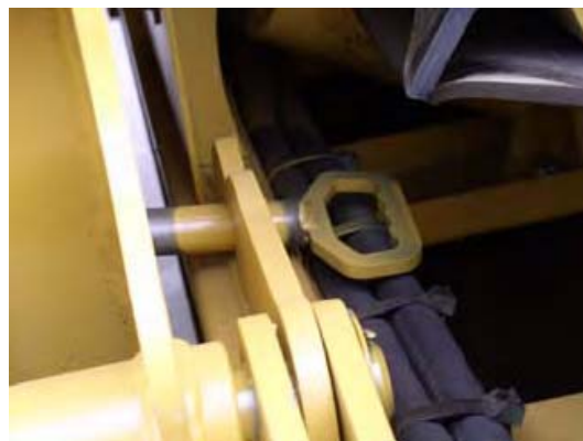
13: Remove mid grade side conveyor bottom section locking pins.
