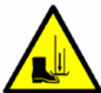
22: Crushing Hazard - Feet
