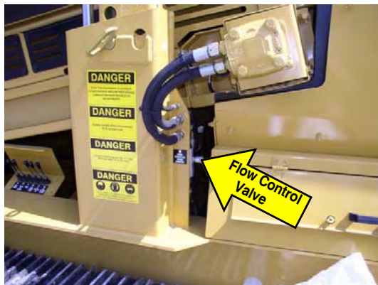
1: Adjusting Fines Collector conveyor speed
