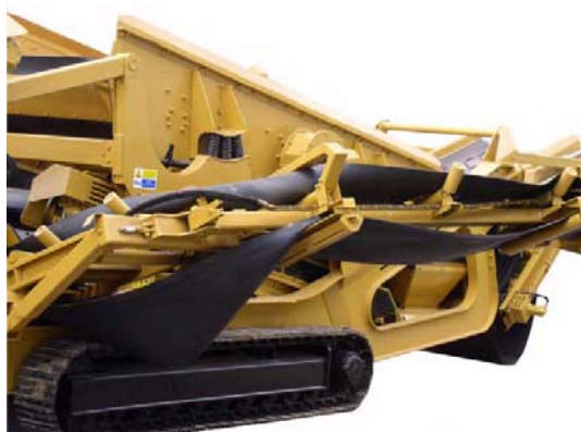
3: R/H Side Conveyor folded down
