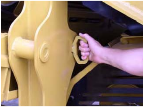
1: Remove mid grade side conveyor bottom section locking pins.
