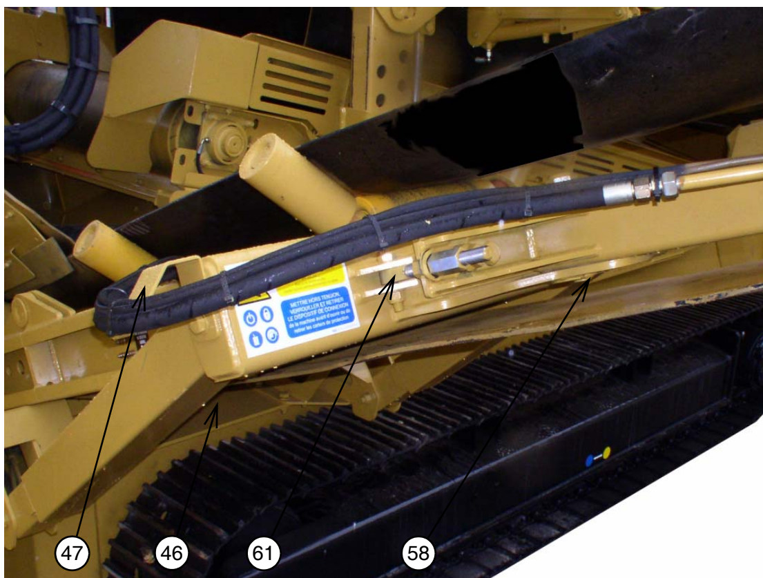
3: FINES SIDE CONVEYOR SPINE PIVOT
