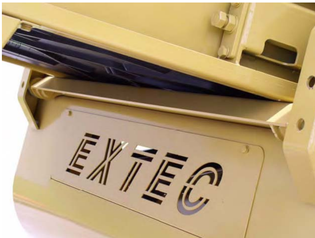
7: Tail Conveyor lowered onto Chassis
