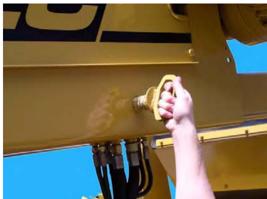
8: Remove locking pins.
