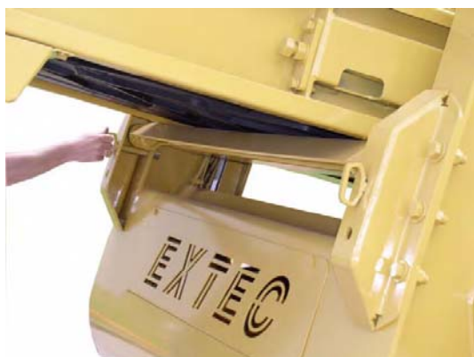
5: Remove pins from underside of tail conveyor.
