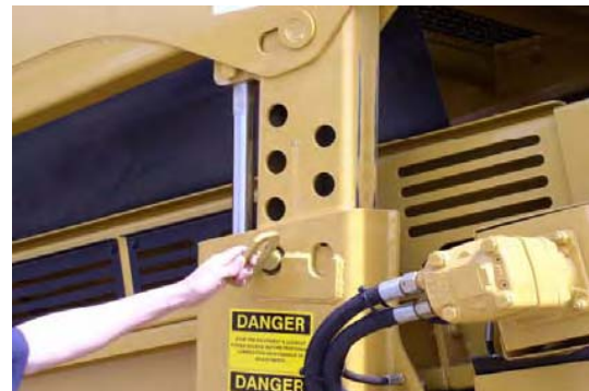
2: Locate pin to lock telescopic leg in raised position.
