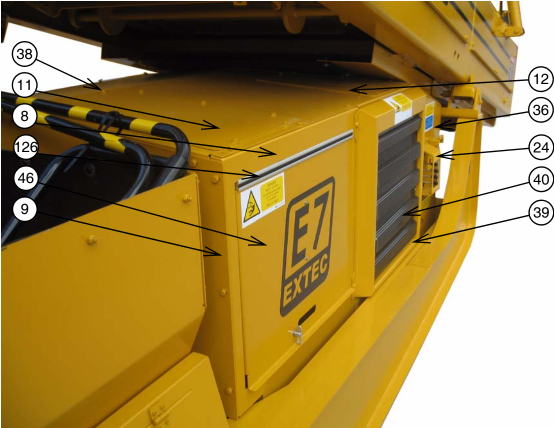
1: VIEW ON L/H SIDE OF POWER PACK
