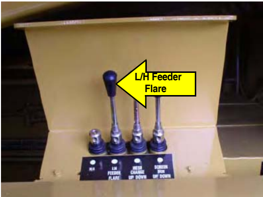
3: Activate 'L/H Feeder Flare' lever.
