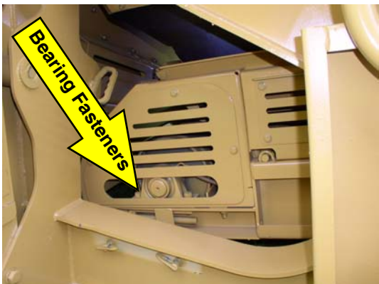
2: Slacken off all tail drum bearing fasteners.
