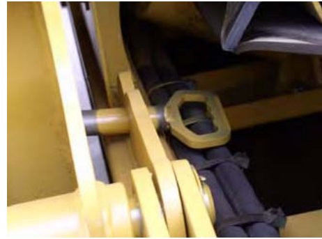
1: Remove mid grade side conveyor bottom section locking pins.
